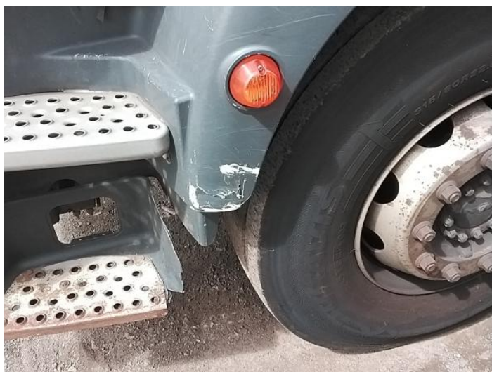
1: Wheel Trim nsf Broken Replace
