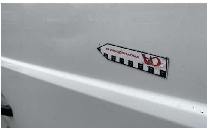
5: Qtr Panel osr Dented Over 30mm
