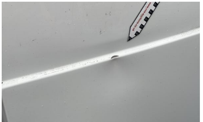
4: Door osf Dented With Paint Damage
